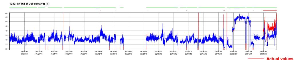
Malfunction detected by mismatch between Al model and real time data
