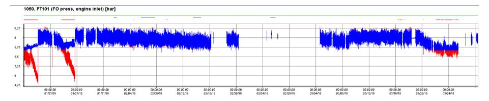
Malfunction detected by mismatch between Al model and real time data
